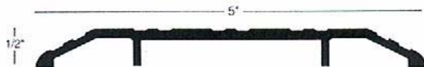
T004 A - B - W - BG #10 x 1-1/2 philips flat head screws are included.
